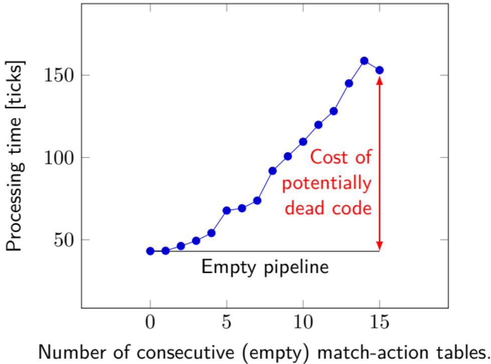
Hand-crafted pipeline as a sequence of JITted empty tables, 10 million packets measured on Intel Core5@2.40GHz CPU/4GB DRAM/Debian/GNU Linux with pmu-tools/jevents.
