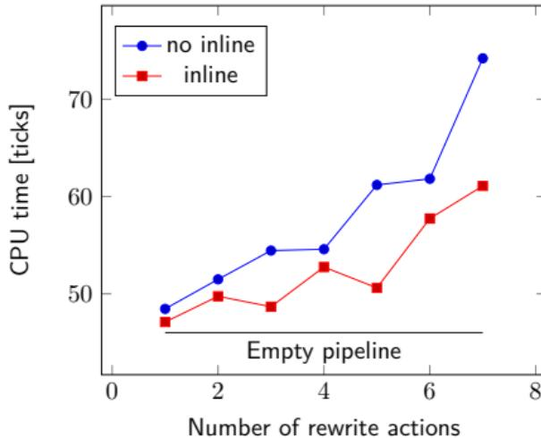
Hand-crafted pipeline with 15 JITted rewrite actions and write templates, 10 million identical packets measured on Intel Core5@2.40GHz CPU/4GB DRAM/Debian/GNU Linux with pmu-tools/jevents.
