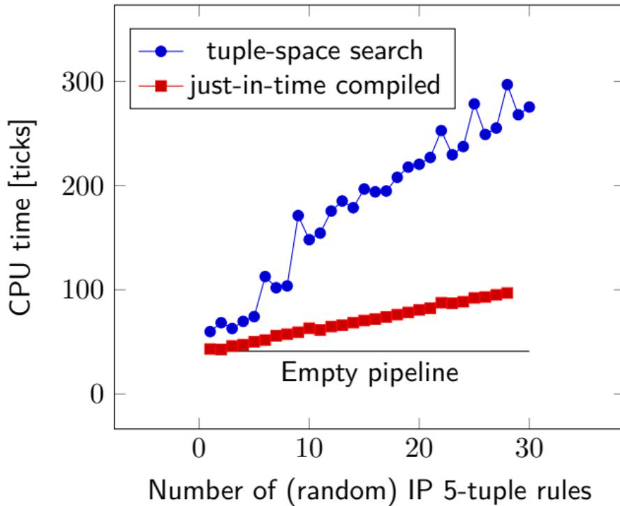
Hand-crafted pipeline with random `match` templates, 10 million identical packets measured on Intel Core5@2.40GHz CPU/4GB DRAM/Debian/GNU Linux with `pmu-tools/jevents`.
