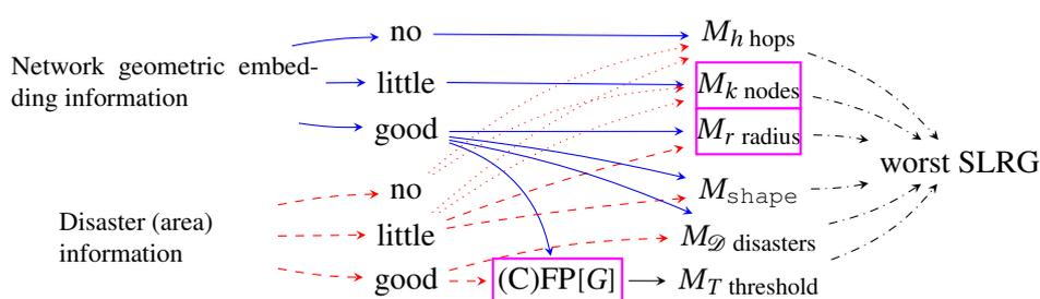
Figure 3.1: A mind map of SRLG and PSRLG problems related to the quality of input data. For a graph  $G$ ,  $(C)FP[G]$  stores PSRLGs, while lists  $M_*$  consists of SRLGs. Problems studied in this Thesis ( $M_k$  nodes,  $M_r$  radius,  $(C)FP[G]$ ) are highlighted with purple rectangles.
