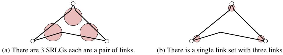
Figure 3.2: Example SRLGs according to (a) Def. 2.1.1, and (b) [42].
