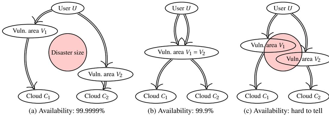
Figure 1.2: User  $U$  reaches his data either in cloud  $C_1$  or in cloud  $C_2$ . At the next disaster, the connections to  $C_1$  and  $C_2$  may fail in regions  $V_1$  and  $V_2$ , respectively, with an equal chance of  $P(V_1) = P(V_2) = 0.001$ . If  $V_1$  and  $V_2$  may be hit by the same disaster, but are not co-located, the cloud availability under the next disaster is hard to estimate.
