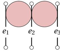
Figure 5.1: In the figure above, the solid circular disks are disasters with radius  $r$ ,  $d(e_1, e_2) = d(e_2, e_3) = 2r$ , while  $d(e_1, e_3) = 4r$ . The set of regional failures is  $F_r = \{\{e_1\}, \{e_2\}, \{e_3\}, \{e_1, e_2\}, \{e_2, e_3\}\}$ . The set of maximal regional failures is  $M_r = \{\{e_1, e_2\}, \{e_2, e_3\}\}$ .
