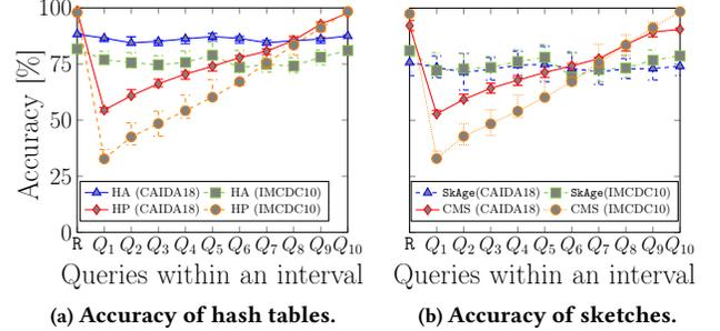
**Figure 1: The impact of QAT on the accuracy within an interval (FI) in the hash table (a) and sketch-based (b) algorithms. 10 queries arrive at every second after the reset (R), each ask for the top-300 HH while the length of the interval-reset algorithm’s intervals, FI is configured to 10 seconds.**
